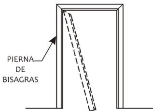
REPETIR PASO #3 CON LA PIERNA DE BISAGRAS. JALAR EL CABEZAL AJUSTANDO SOBRE LAS PERNAS. TRABE EL CABEZAL Y LAS PERNAS DOBLANDO LAS LENGÜETAS EXPUESTAS
